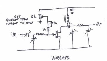
A VN88AFO Replaces the 25C1206 (which does not have sufficient gain at ? This provides about 1-2 w output to the final Linear stage.
