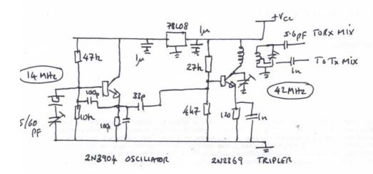
The above circuit replaces the single oscillator @ 22 MHz in the original design to provide 42 MHz to the wixer.
